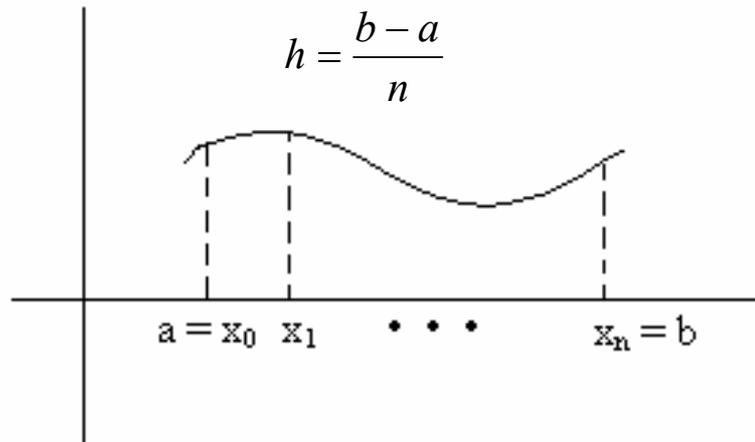
$$I = \int_{x_0}^{x_n} f(x) dx = \int_{x_0}^{x_1} f(x) dx + \int_{x_1}^{x_2} f(x) dx + \dots + \int_{x_{n-1}}^{x_n} f(x) dx$$
