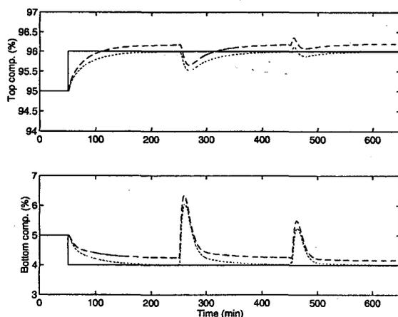
Figure 10. Responses of the PCR model based inferential feedback controllers without mean updating
