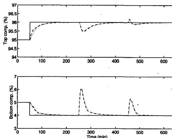
Figure 11. Responses of the PCR model based inferential feedback controllers with mean updating
