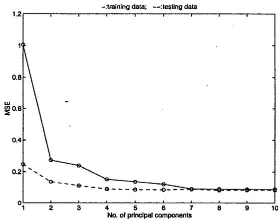
Figure 4. Mean squared errors of different PCR models
