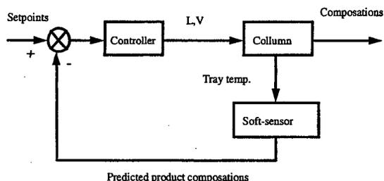
Figure 8. Inferential feedback control structure
